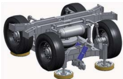
DCC's new generation of vehicles uses the vehicle bogie in a Jacob's arrangement
